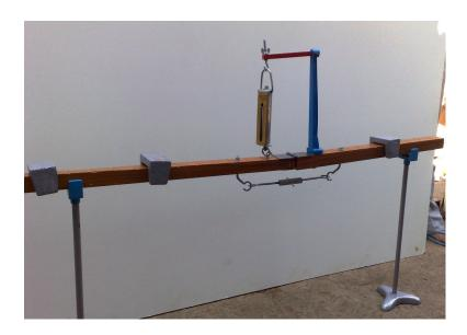
Apparatus consists of two knife edge supports on stands and a bar 180cm long which is hinged at one point of its length. The dynamometer with an adjusting screw for restoring line of beam under load conditions is supplied with the apparatus. Apparatus is supplied complete with three sliding 'U' shaped weights.
